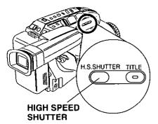
Press <u>HIGH SPEED SHUTTER</u> while recording.
