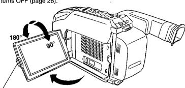
Press <u>LCD-OPEN</u> to unlock the LCD monitor. Swing it fully open and adjust the angle.
