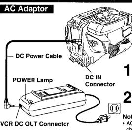
Connect AC Adaptor VCR DC OUT to Camcorder DC IN with supplied DC Power Cable.
